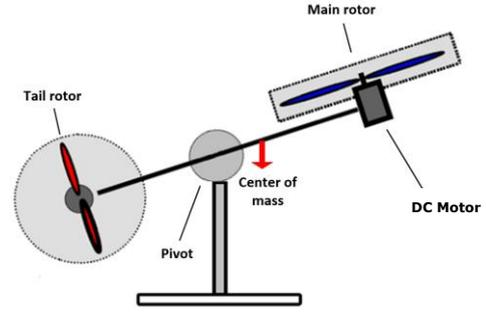
Figure 1. Aerodynamic model of the helicopter system.
