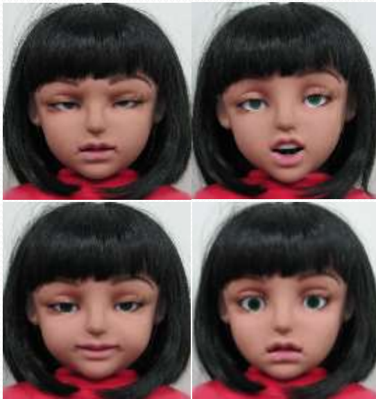
Mina humanoid robot ( R50 Alice ) with ability of producing human facial gestures
