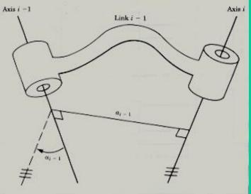
2 Angle between lines measured in the plane whose normal is the common normal. This angle is called the "Link-Twist"(پيچش رابط), α<sub>i-1</sub> measured from axis i-1 to axis i by Right-Hand-Rule about the common normal. Note: If the axes intersect, then a is zero, and α is still measured from axis i-1 to axis i.
