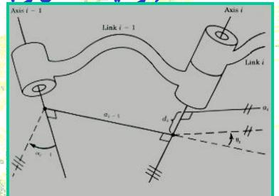
For Prismatic Joints: a,  $\alpha$ , and  $\theta$  are all fixed, then "d<sub>i</sub>" is the Joint Variable (متغير مفصلى).
